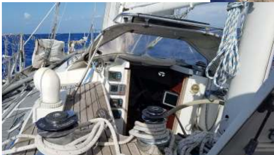
View of center cockpit. This unusual boat design had two cockpits! The rear one was very conventional looking except no wheel to steer by. Note wheel attached to rear wall of cockpit. Thankfully the autopilot did all of the steering.
